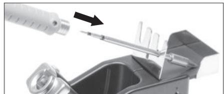
Insert the new cartridge\* and press slightly as far as the mark and tighten the screw.
