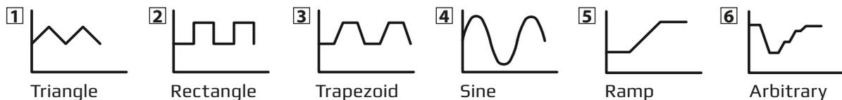
Additionally to the standard functions, which are all based upon a so-called arbitrary generator, this base generator is accessible for the creation and execution of complex sets of functions, separated into up to 99 sequences. Those can be used for testing purposes in development and production. The sequences can be loaded from and saved to a standard USB stick via the USB port on the front panel, making it easy to change between different test sequences.
