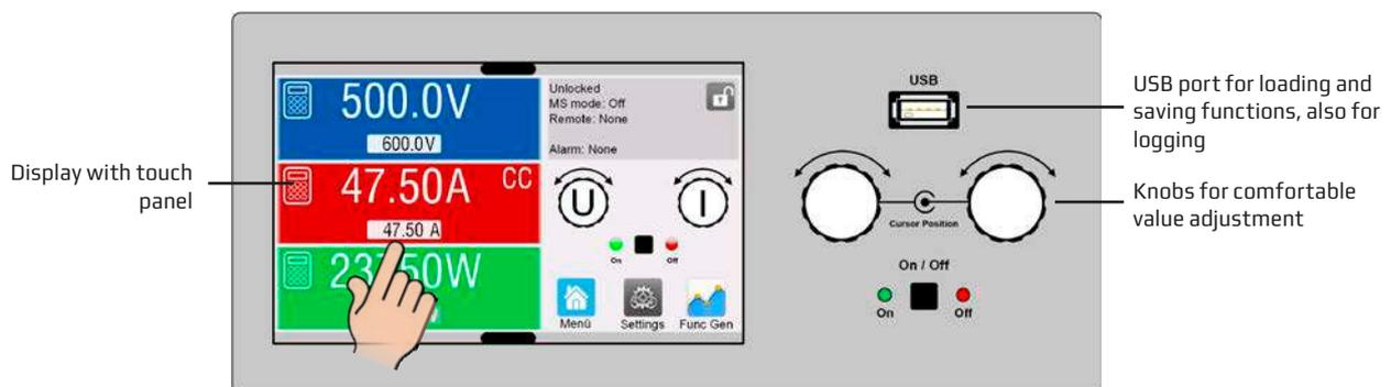
Set values and actual values of output voltage, output current and output power are clearly represented on the graphic display. The color TFT screen is touch sensitive and can be intuitively used to control all functions of the device with just a finger tip.
