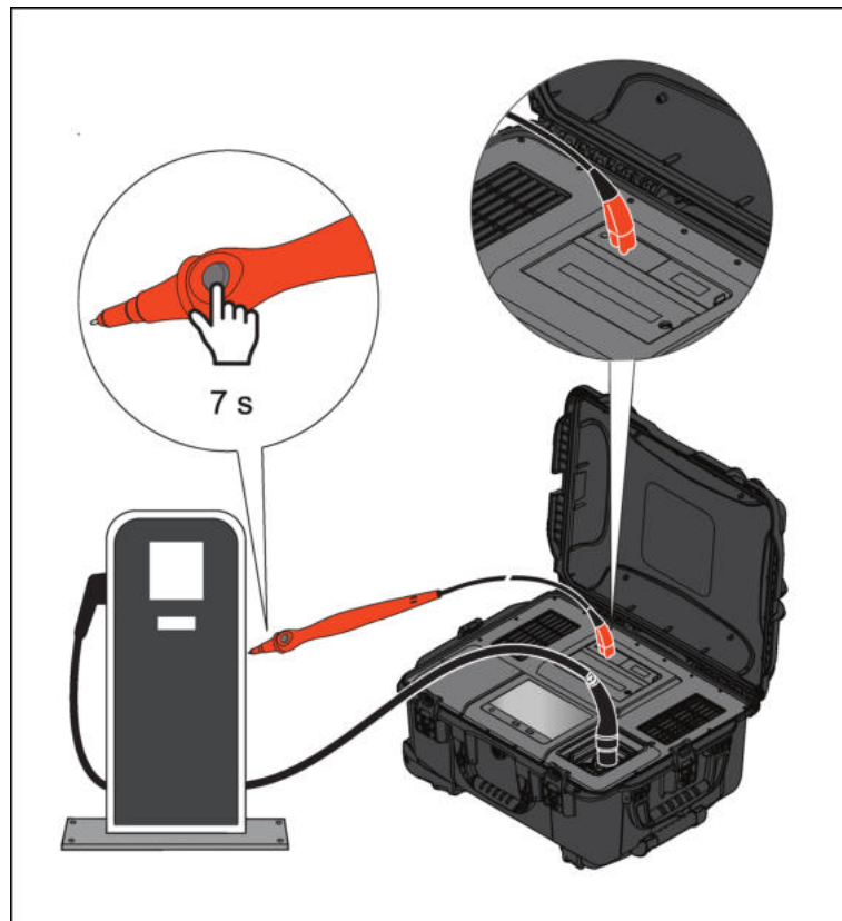
Figure 5. Performing Continuity Test
