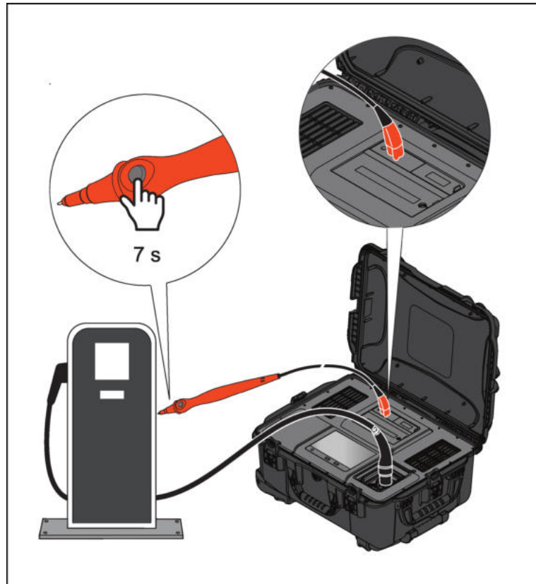
Figure 5. Performing Continuity Test
