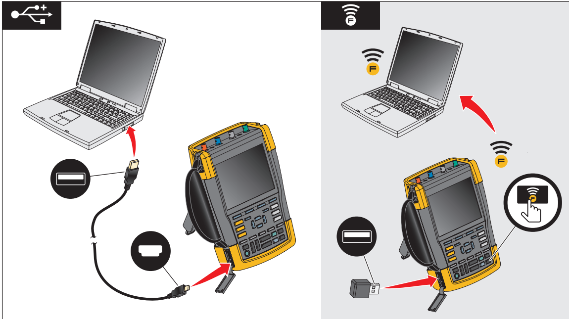
Figure 1. Test Tool to PC Connections
