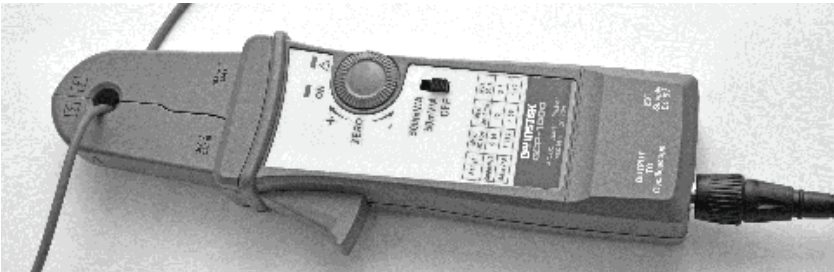
Figure 2. Connecting the GCP-1000 current probe.
