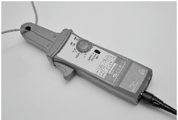
Figure 2. Connecting the GCP-300 current probe.
