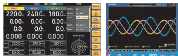
AC Unbalanced Three-phase
