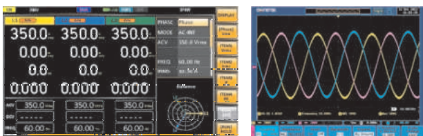
AC Balanced Three-phase
