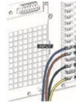
AC Three-phase Input (Y Connection)
