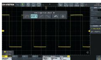
The AUTOSET Button Automatically Identifies Waveforms
