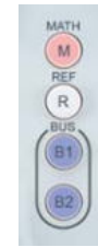
The GDS-3000 Series provides two dedicated keys in the front panel for two sets of setting recall
