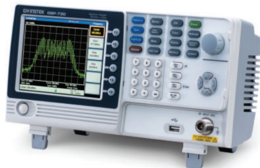
Figure A-2. Reference platform: GSP-730 Spectrum Analyzer
