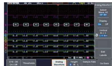
Display analog waveform converted from digital signal
