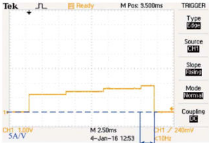
Over current protection time is about 2.015ms
