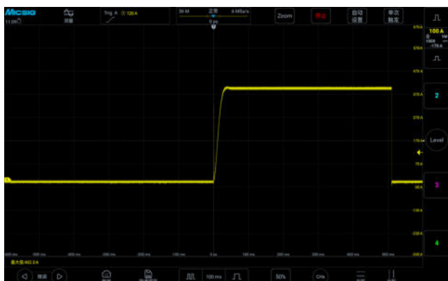
CP3008: Accurate transient capture for 400 A high-current signals.
