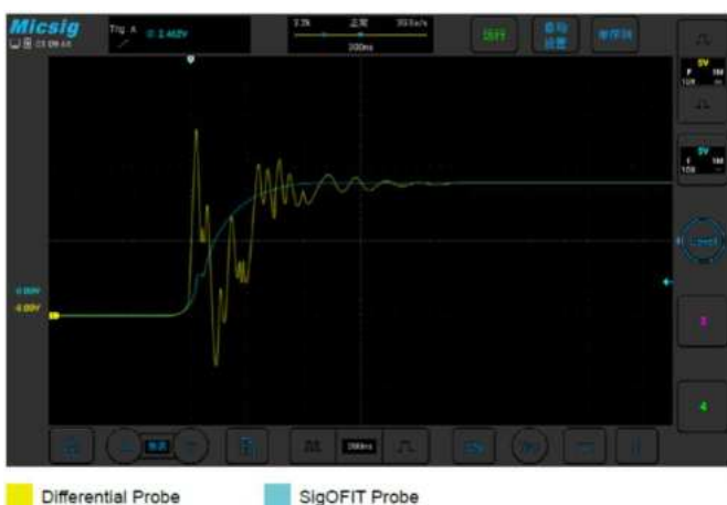
▲ Vgs signal at SiC conduction moment
