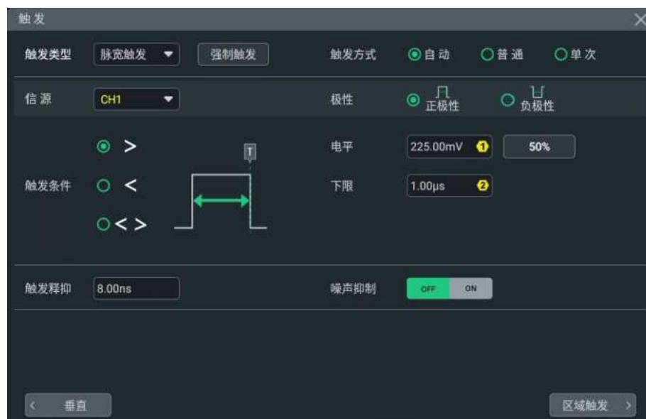
Figure 8.5 Pulse Trigger Setting Menu
