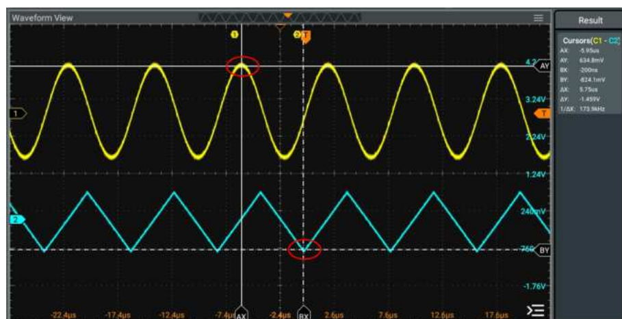
Figure 10.9 Track Measurement (before Horizontal Expansion)
