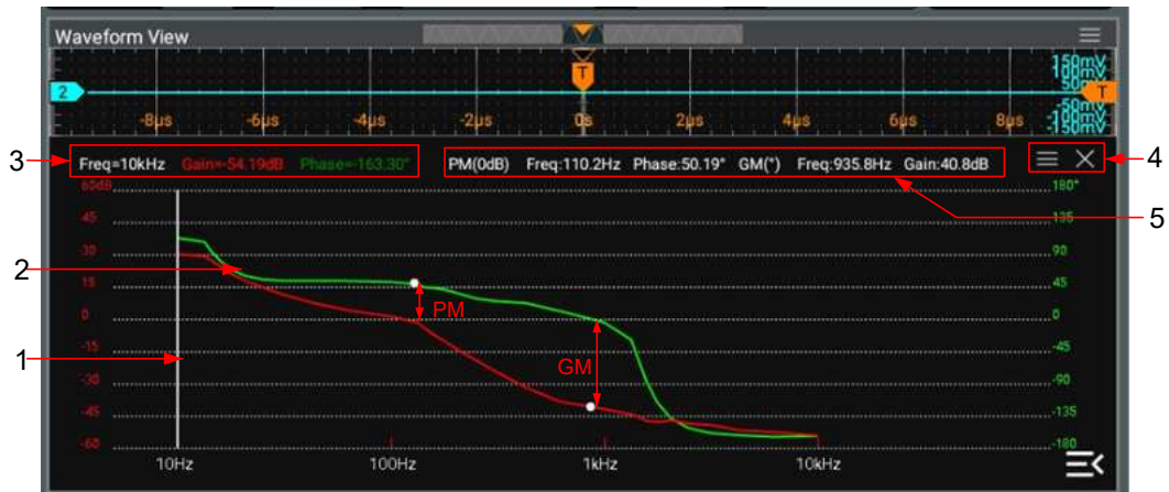
Figure 15.3 Bode Plot Waveform Display
