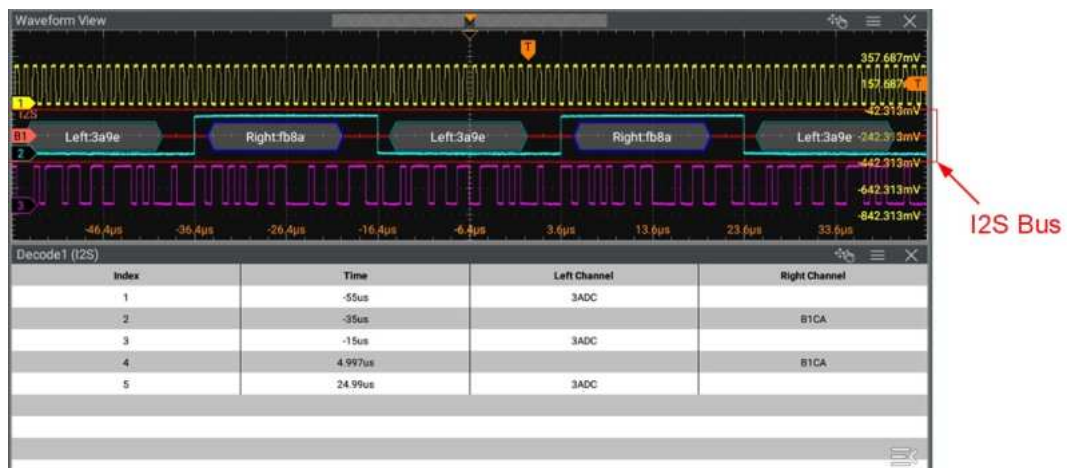
Figure 19.19 I2S Decoding Event Table
