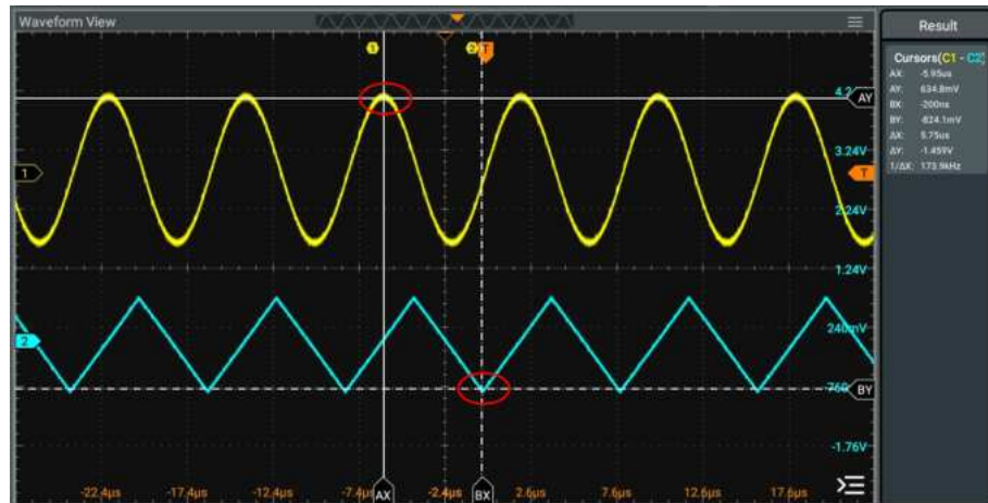
Figure 10.10 Track Measurement (after Horizontal Expansion)
