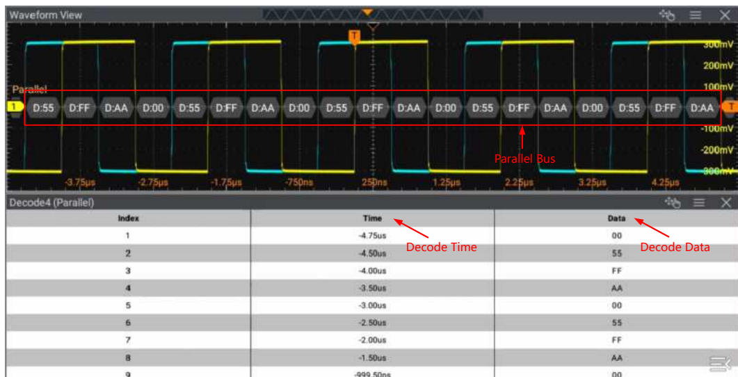
Figure 19.3 Parallel Decoding Event Table
