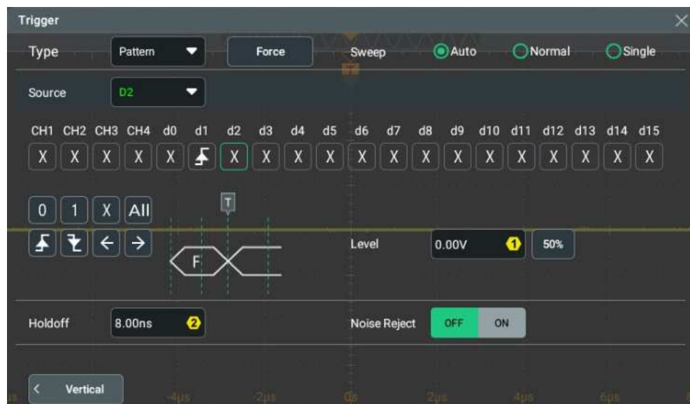
Figure 8.10 Pattern Trigger Setting Menu
