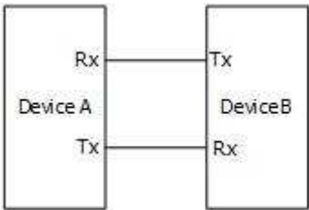
Figure 18.4 Schematic Diagram of RS232 Serial Bus
