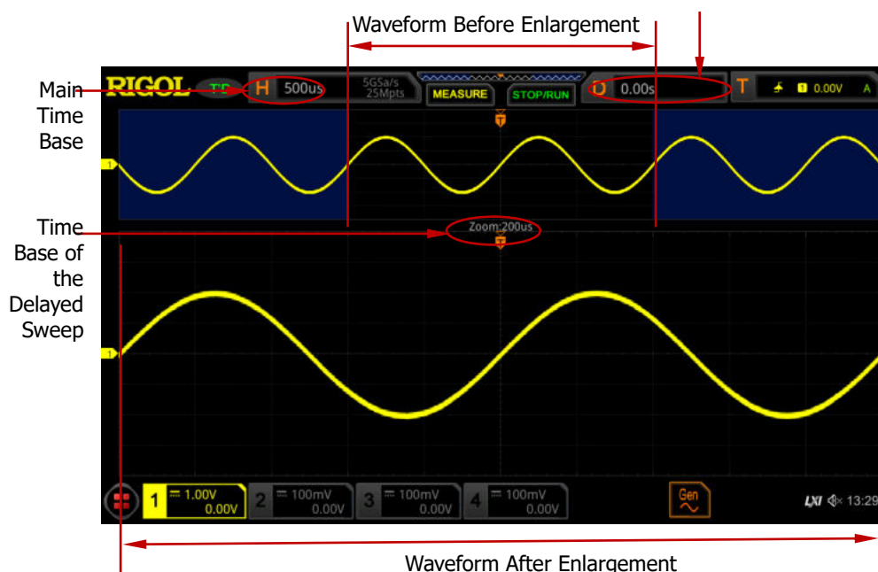
Figure 3-1 Delayed Sweep Mode
