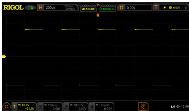
Figure 4-3 Waveforms after 128 Times of Averaging
