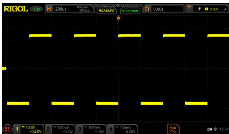
Figure 4-2 Waveforms before Averaging
