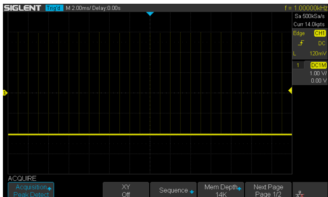
Figure 21 Pulse With 0.1% Duty, Peak Detect Mode
