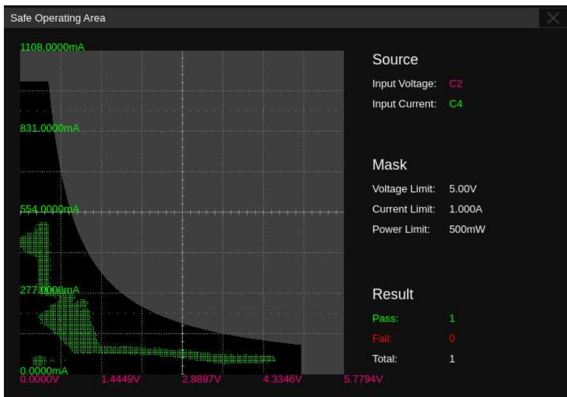
Voltage and current waveforms on the MOSFET at power-up
