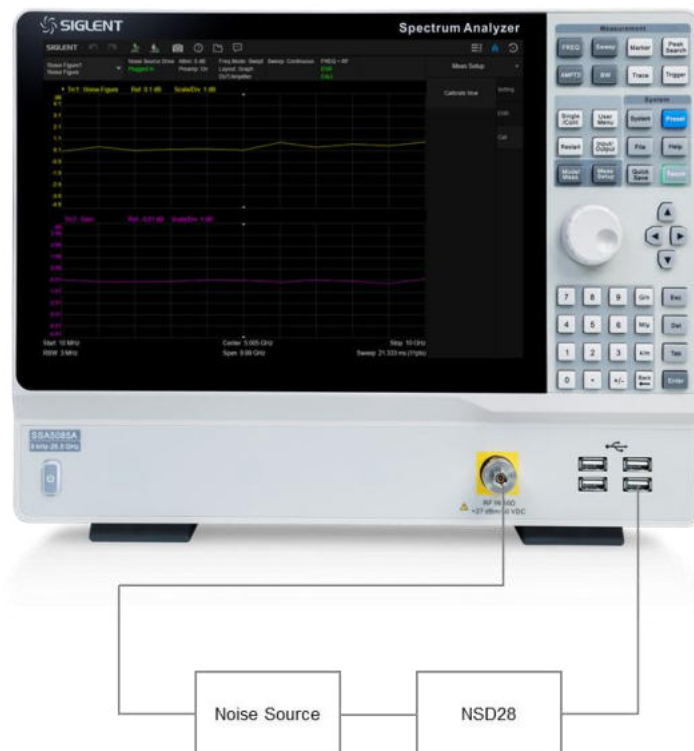
Figure 1-2 Connection setting of noise figure measurement calibration
