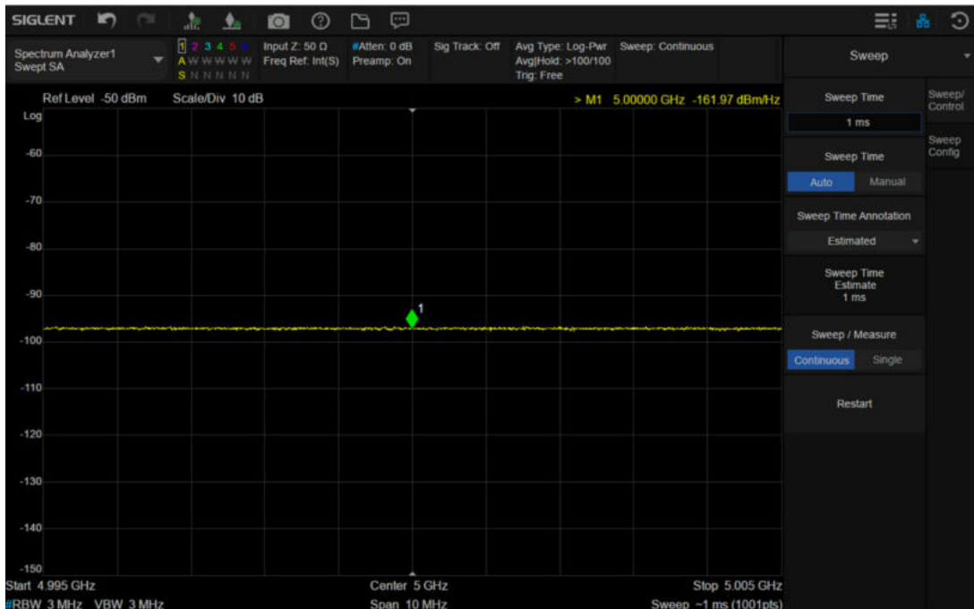
Figure 1-9 Noise power spectral density of unconnected power supply
