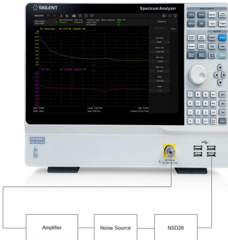
Figure 1-6 Connection settings for noise figure measurement
