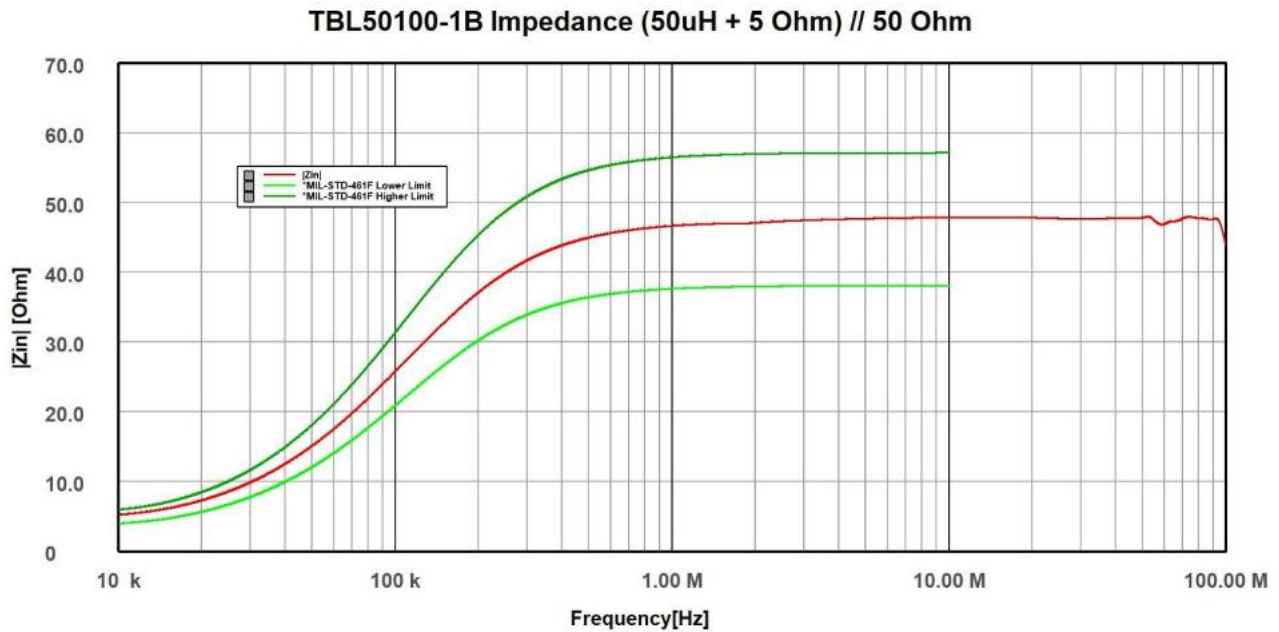
Picture 3: LISN impedance, (50 \mu H + 5 \Omega ) // 50 \Omega MIL-STD
