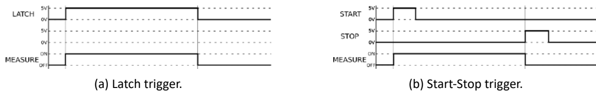
Figure 9.8: SMARTIS trigger options - Latch or Start-Stop triggers.
