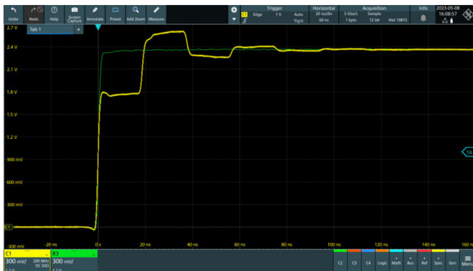
Screenshot: Reflections on non-terminated lines
