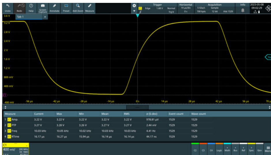
Screenshot: Automatic measurement of various signal parameters
