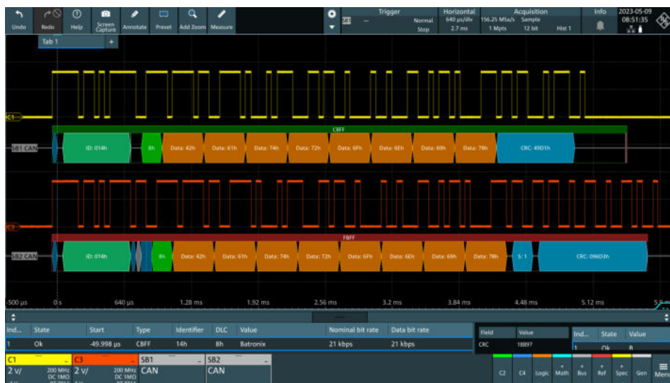
Screenshot: CAN interface decoding and decoder table
