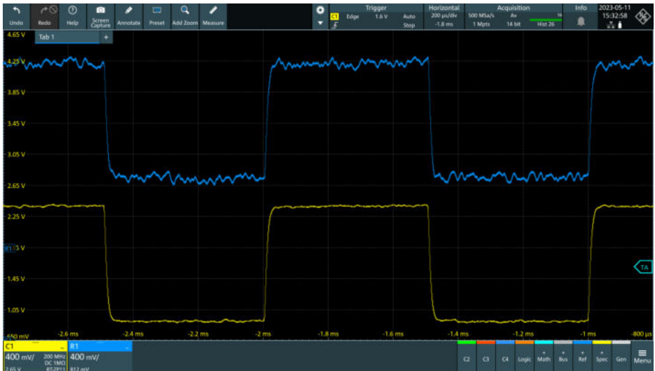
Screenshot: 1 kHz square wave with strong noise (blue reference: normal mode, yellow signal: average mode)
