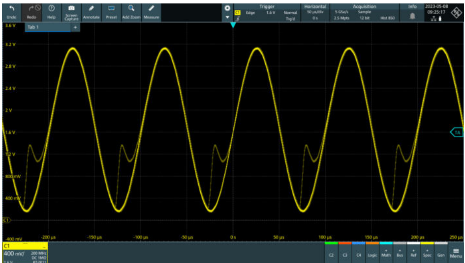
Screenshot: Better visibility of rare signal events by setting the display persistence
