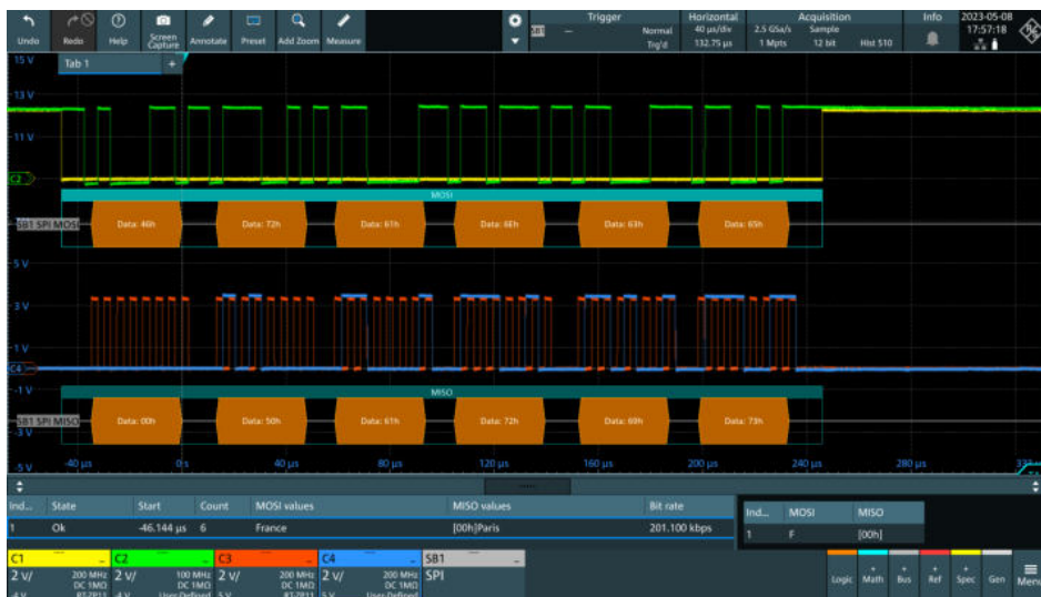
Screenshot: SPI interface decoding and decoder table
