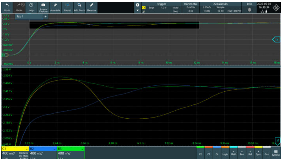
Screenshot: Signal influence due to loading with a probe
