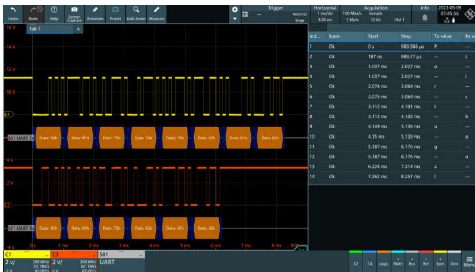
Screenshot: UART interface decoding and decoder table
