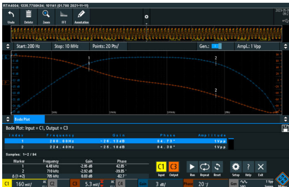
Screenshot: The Bode plot of the demonstration filter on the demo board
