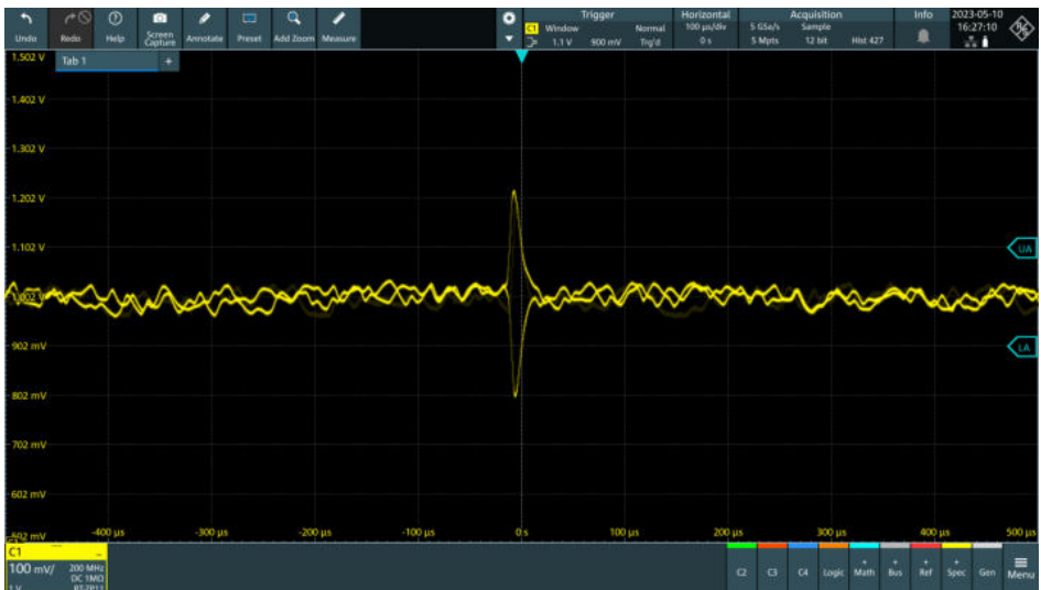
Screenshot: Triggering with the window trigger on positive and negative peaks of a power supply line
