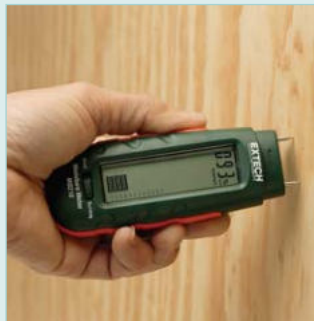
Quick measurement of Moisture levels on wood and building materials.
