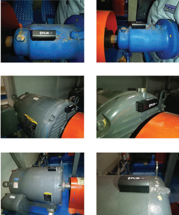
Figure 6.2 SV87 sensors shown mounted on machinery.
