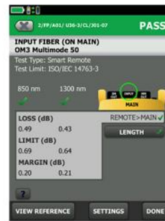
Detail shows margin and allowable limits for the fiber at two wavelengths.
