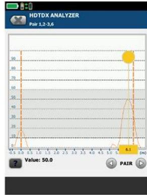
High Definition Time Domain Cross talk (HTDTX) shows the far end connection is clearly the issue
