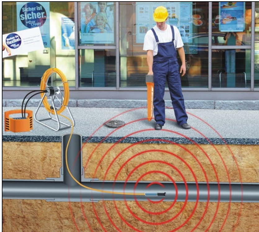
Fig. 9: Signal coupling in non-metallic pipes
