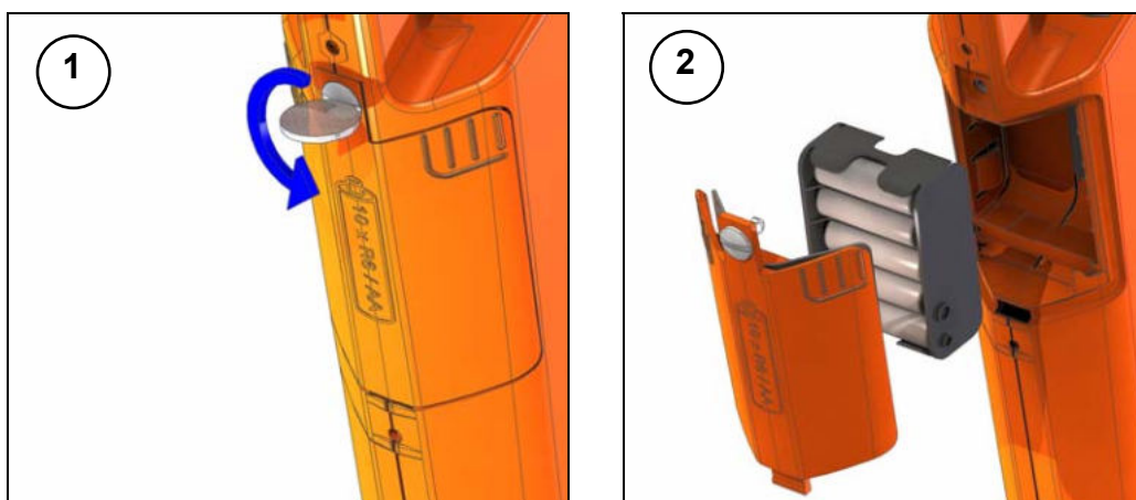
Fig. 15: Replacement internal batteries of RX5000
