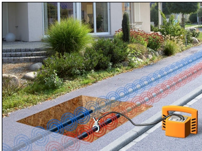
Fig. 6: Coupling via transmitter clamp
