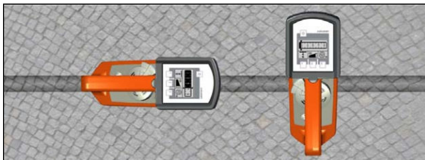
Fig. 12: Alignment of the receiver RX5000
