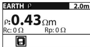
Fig. 29: Result screen of ground resistance measurement
