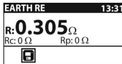
Fig. 26: Result screen of earth resistance measurement
