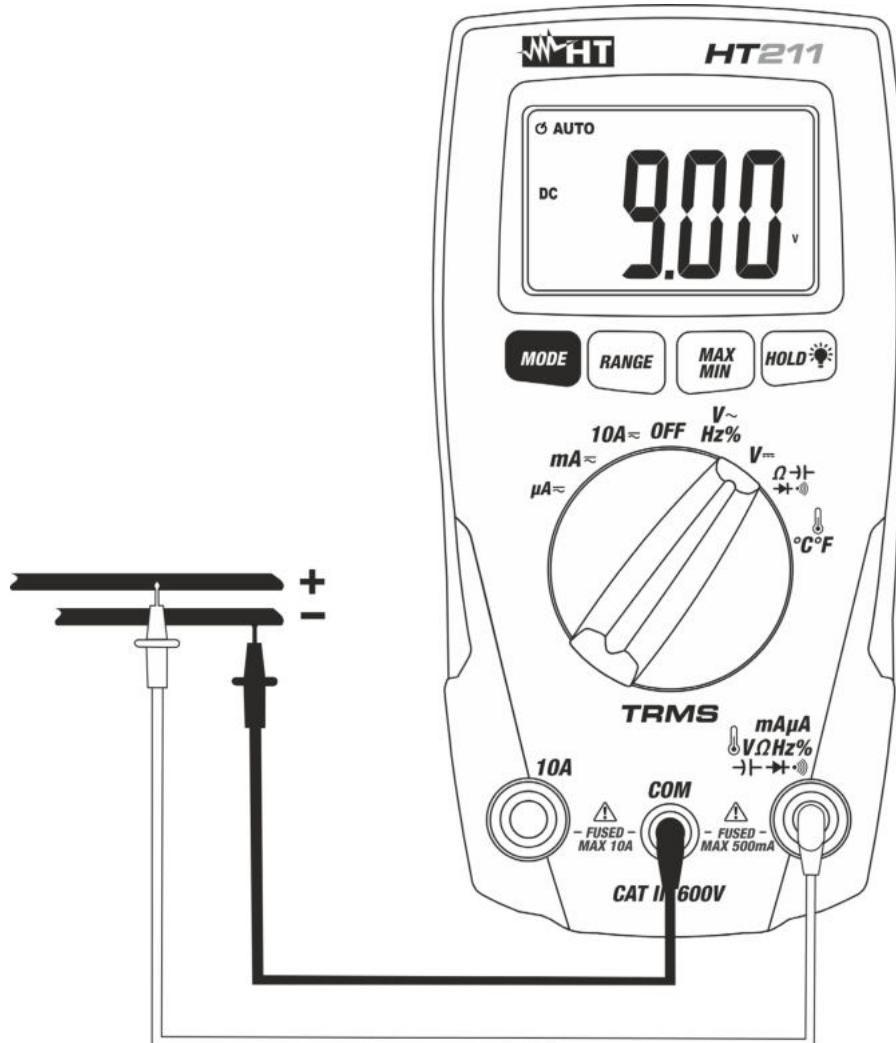
Fig. 2: Using the meter for DC Voltage measurement
