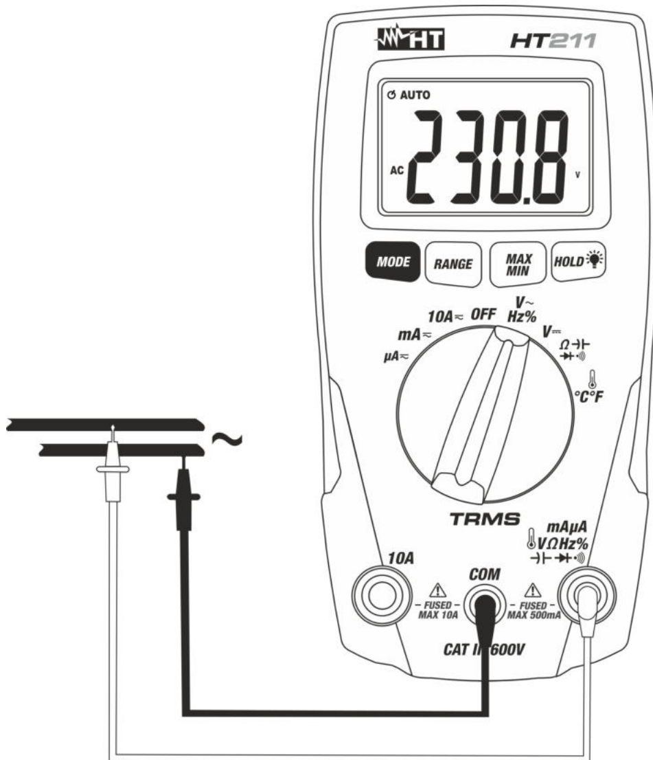
Fig. 3: Using the instrument for AC Voltage measurement
