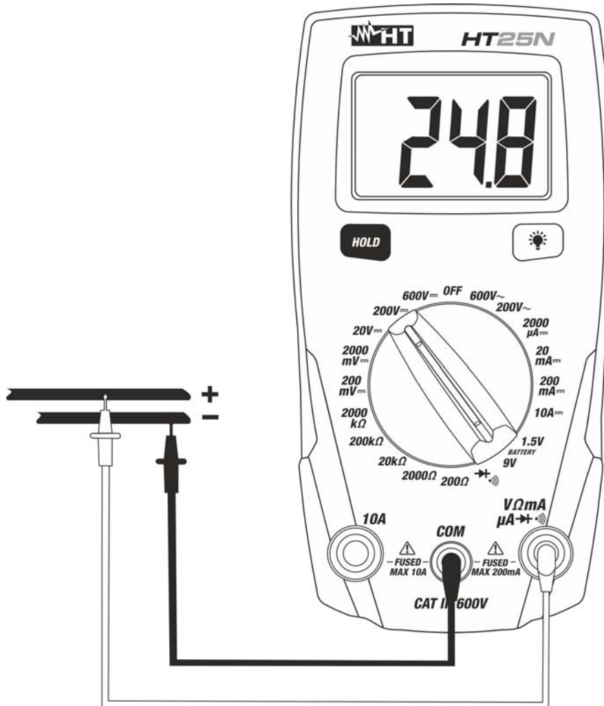
Fig. 2: Using the meter for DC Voltage measurement
