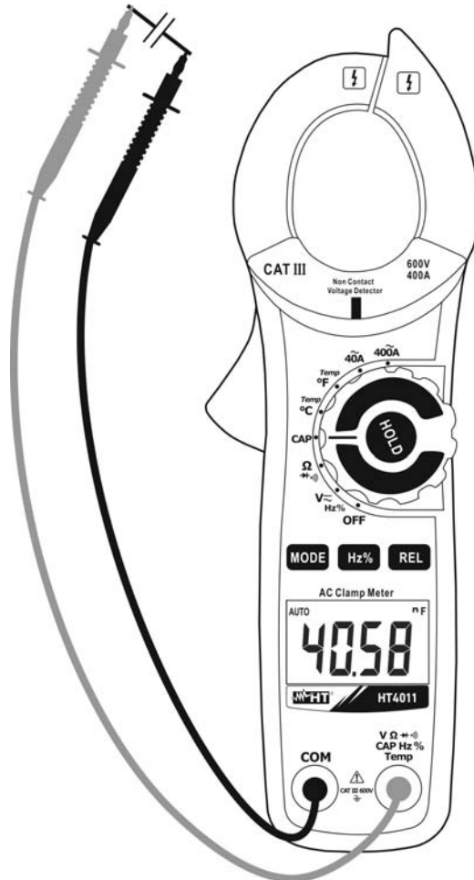
Fig. 6: Use of the clamp for capacitance measurement
