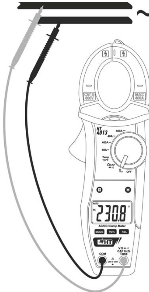
Fig. 4: Use of the clamp for AC voltage measurement
