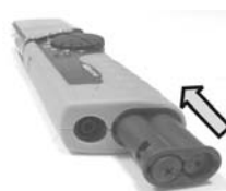
Fig. 8: Opening and closing of battery cover
