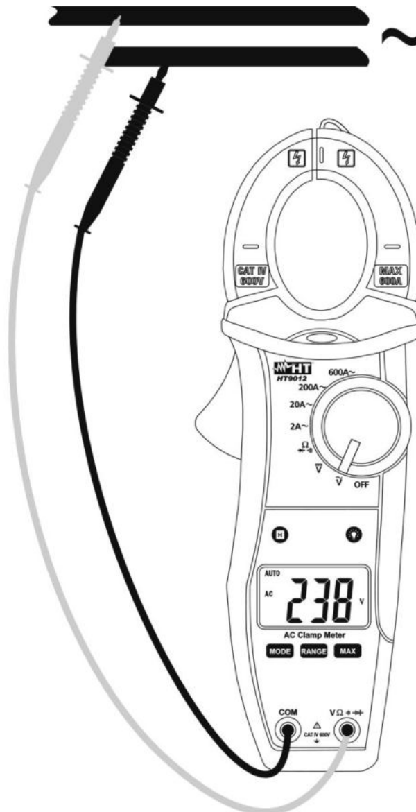
Fig. 4: Taking AC voltage measurement
