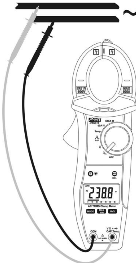
Fig. 3: Taking AC voltage measurements
