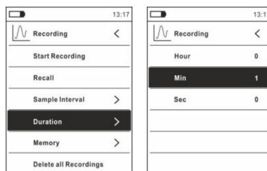
Fig. 36: Data logger function – Setting of recording duration
