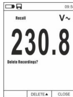
Fig. 40: Data logger function – Deleting recorded data
