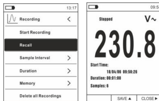
Fig. 38: Data logger – Recalling recorded data to the display
