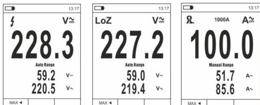
Fig. 6 Description of AC+DC Voltage and Current measurement
