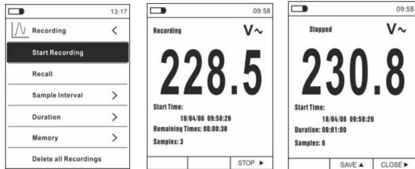
Fig. 37: Data logger function – Starting and stopping recording
