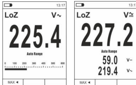
Fig. 10 Description of LoZ voltage measurement
