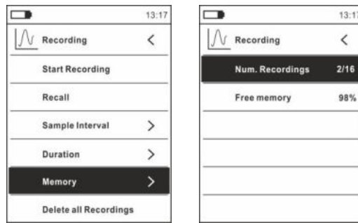
Fig. 41: Data logger function – Content of the memory
