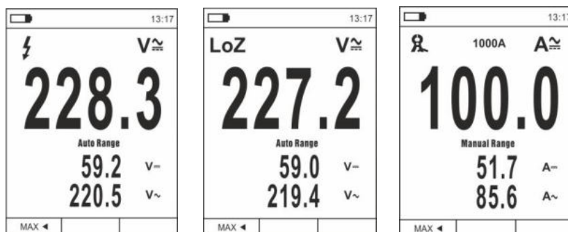
Fig. 6 Description of AC+DC Voltage and Current measurement
