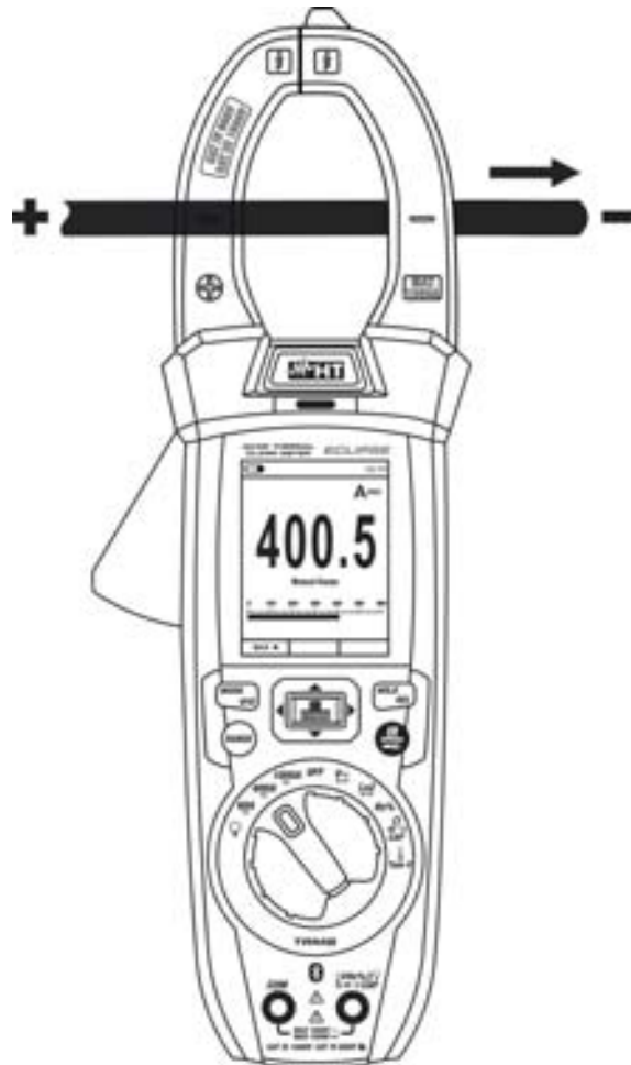
Fig. 31: Use of the instrument for DC current measurement
