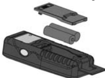
Fig. 14: Replacement of the internal battery
