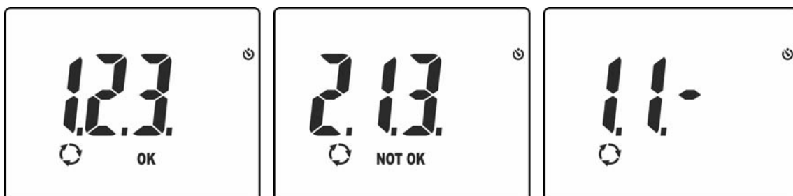
Fig. 16: Results of phase sequence and phase concordance test
