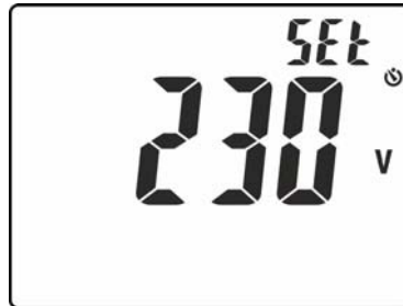
Fig. 6: Setting the rated voltage in Loop measurement
