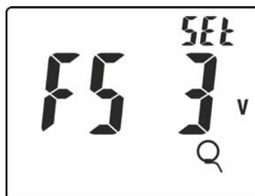
Fig. 7: Setting full scale of flexible clamp
