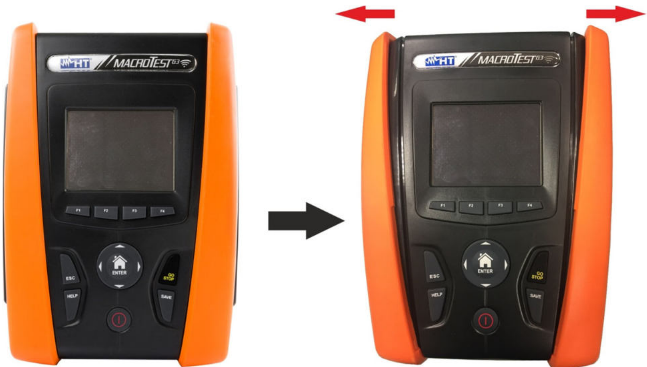
Fig. 40: Remove lateral half-shells
