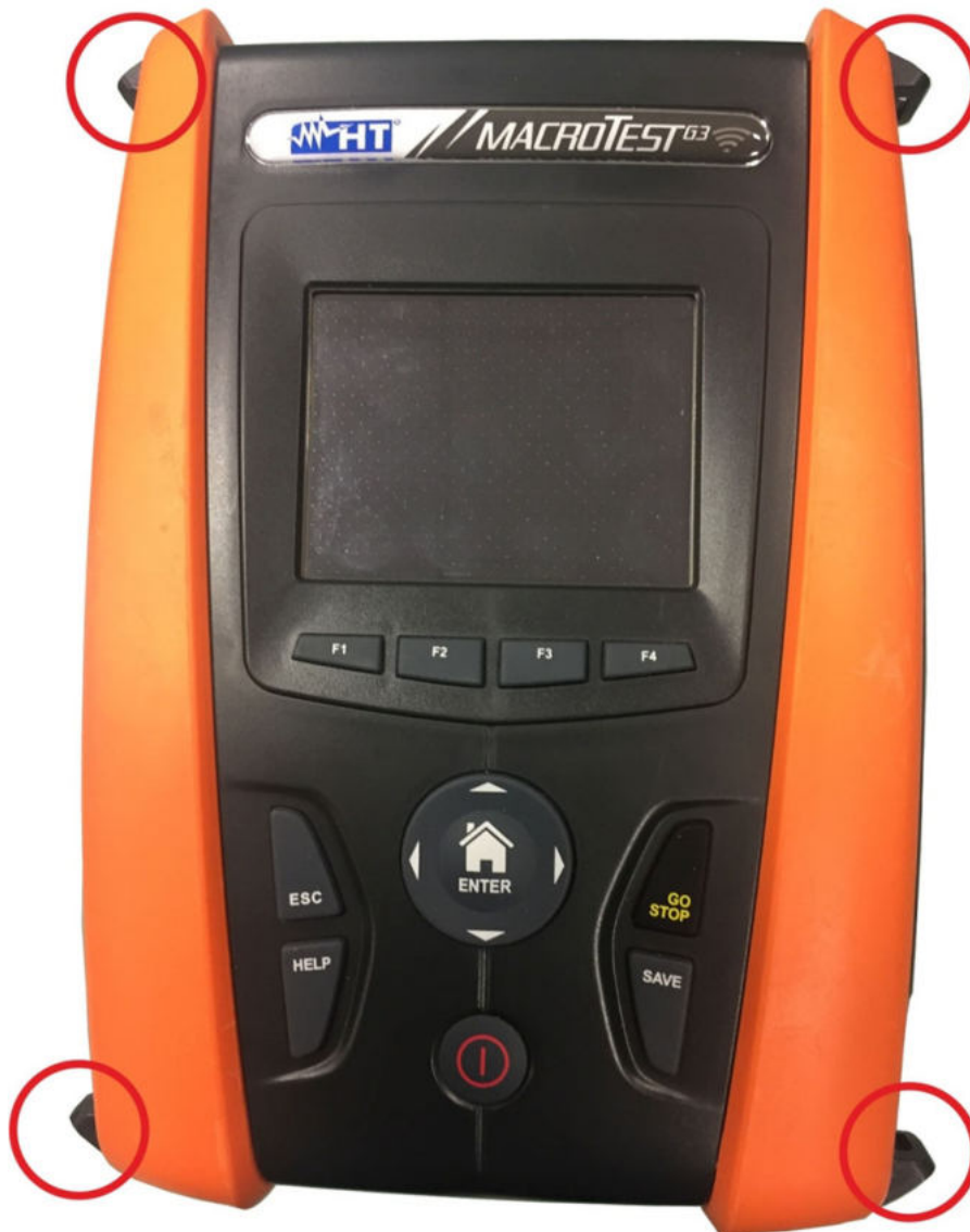
Fig. 42: Instrument with fitted half-shells and hooks
