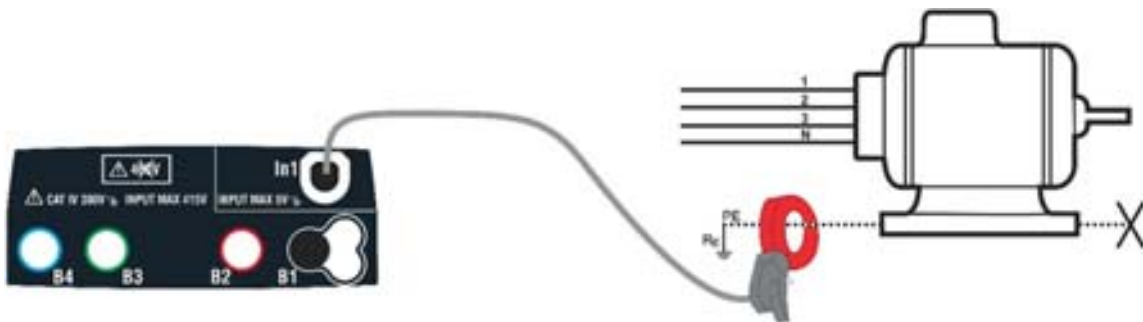
Fig. 27: Direct measurement of leakage current in three-phase systems
