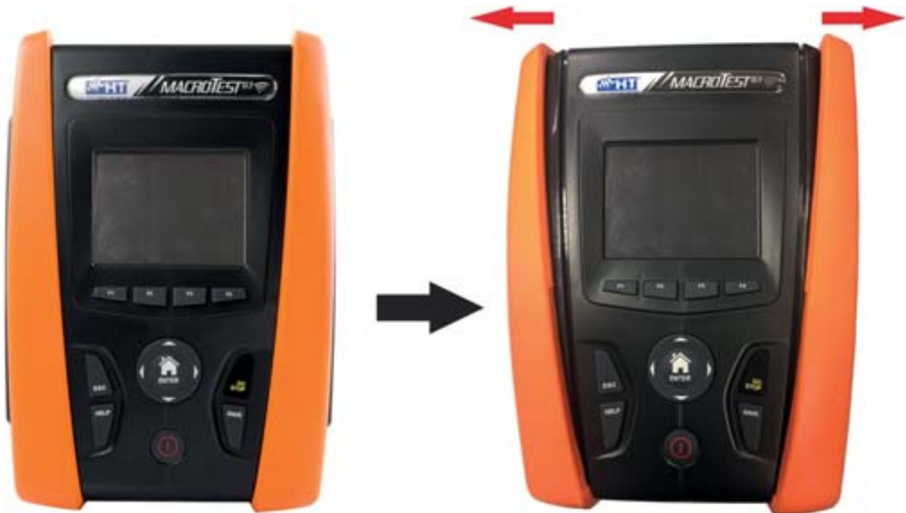
Fig. 40: Remove lateral half-shells
