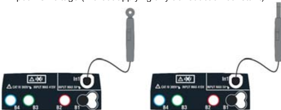
Fig. 33: Measurement of environmental parameters through external probes
