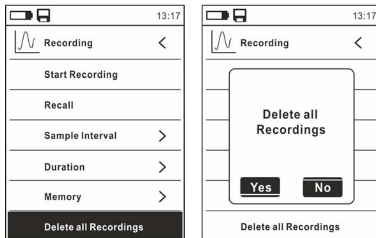
Fig. 38: Data logger function – Deleting all recordings
