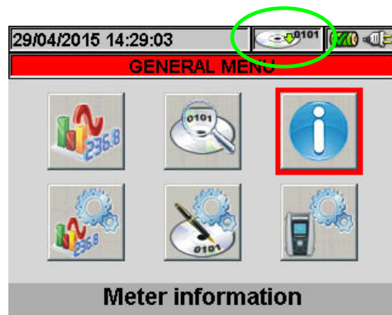
Fig. 87: Meter in recording run
