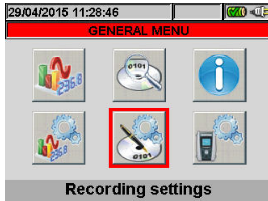
Fig. 63: Recording Settings screen selection
