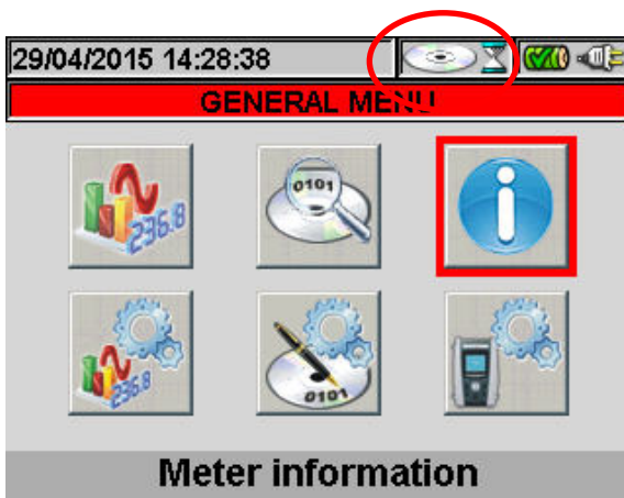
Fig. 86: Meter waiting for recording
