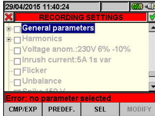
Fig. 66: General Parameters section: no selection
