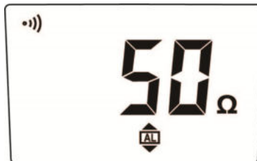
Fig. 33: Setting of alarm thresholds in resistance measurement
