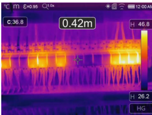
Distance measurement with laser pointer
