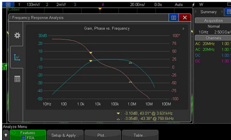
Figure 23. Frequency response analysis plot (Bode gain & phase) of a bandpass filter.
