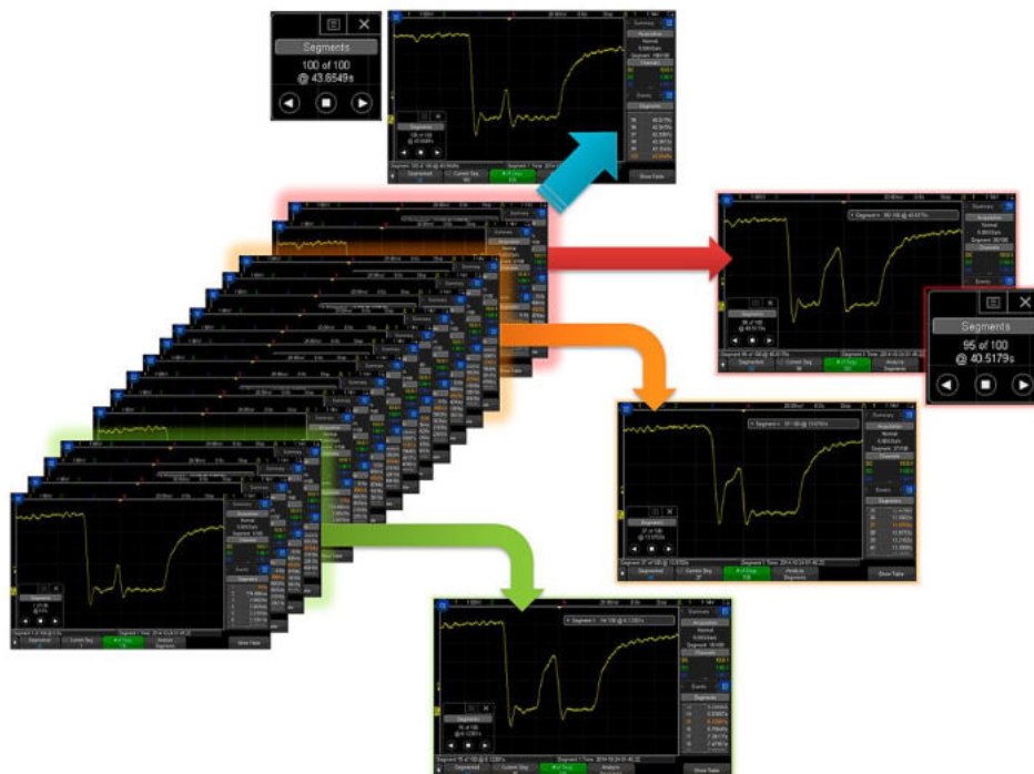
Figure 13. Segmented memory reveals different types of glitches are taking place.
