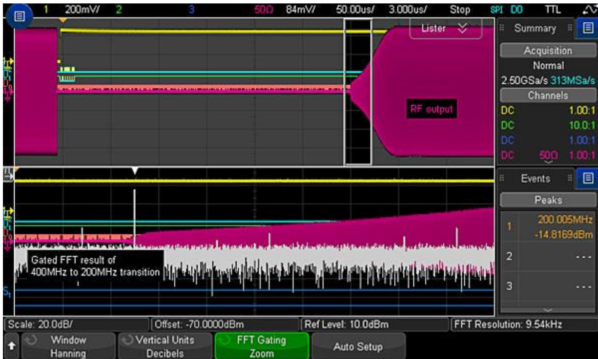
Figure 21c. Start observing the RF signal at 200 MHz. You can validate this from the RF analog waveform as well.
